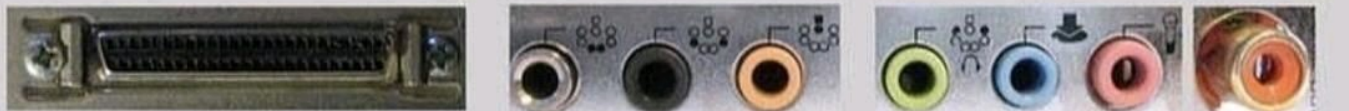
50 pin SCSI 2 Surround sound stereo/Headphones Line In Mic Digital Audio RCA plug style
