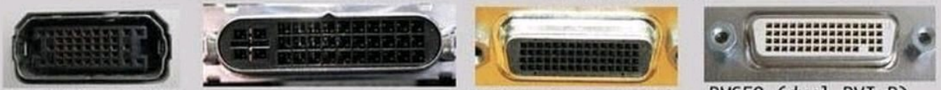
Apple Hi-Density Video HDI-45 Apple Display Connector - ADC LFH60 (dual DVI-D) DMS59 (dual DVI-D)
