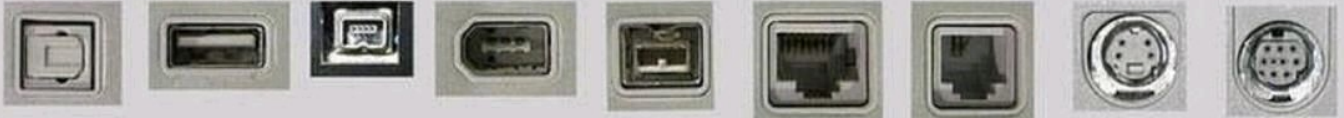
Optical Audio "Toslink" USB A 1.0/1.1/2.0 Firewire 4 pin iLink Firewire 400 1394a Firewire 800/3200 1394b/c Ethernet 8P8C common:RJ-45 Modem RJ-11 Apple Desktop Bus - ADB Mac Serial
