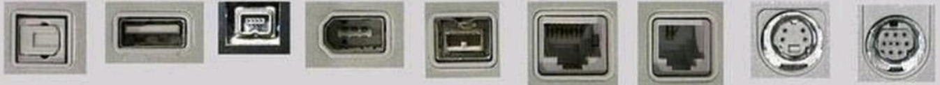
Optical Audio "Toslink" USB A 1.0/1.1/2.0 Firewire 4 pin iLink Firewire 400 1394a Firewire 800/3200 1394b/c Ethernet 8P8C common:RJ-45 Modem RJ-11 Apple Desktop Bus - ADB Mac Serial
